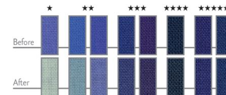
An 8-point scale used to measure the lightfastness of colours based on their degree of fading after exposure to light. A lightfastness rating of between \*\* and \*\*\*\*\* has been determined for the 84 colours of our Pastel Pencils.
